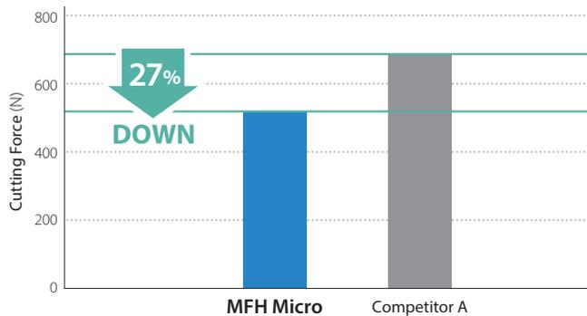
Cutting Conditions:  $V_c = 120$  m/min,  $f_z = 0.6$  mm/t,  $a_p = 0.4$  mm
