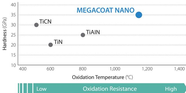
Achieve long tool life with the combination of a tough substrate and a special Nano coating layer
