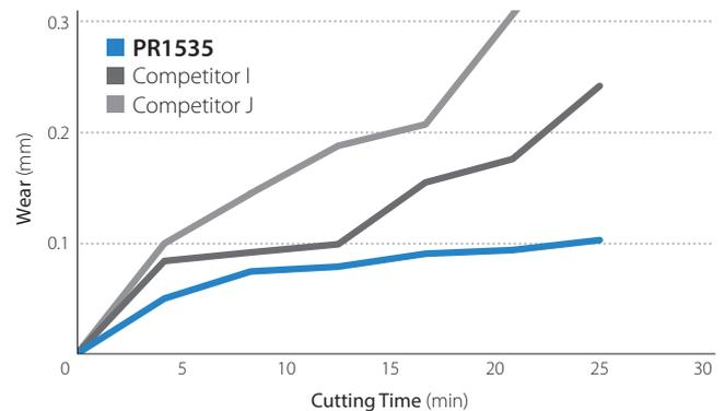
Cutting Conditions:  $V_c = 180$  m/min,  $f_z = 0.5$  mm/t,  $a_p \times a_e = 0.3$   $\times$  8 mm
