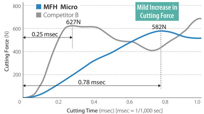
Cutting Conditions:  $V_c = 120$  m/min,  $f_z = 0.6$  mm/t,  $a_p \times a_e = 0.4 \times 5$  mm
