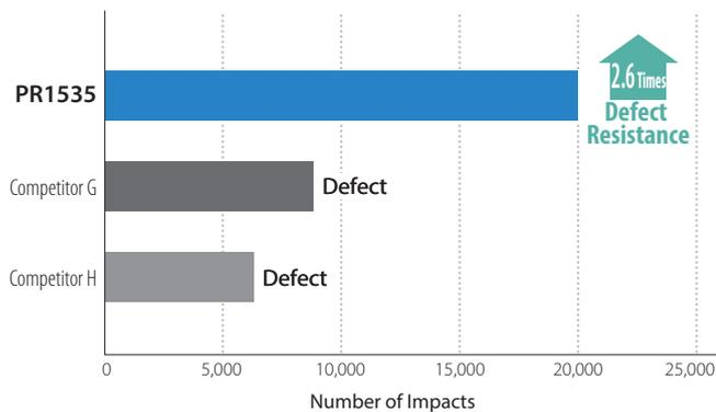
Cutting Conditions:  $V_c = 120$  m/min,  $f_z = 1.5$  mm/t,  $a_p \times a_e = 0.4$  mm  $\times$  2.5 mm
