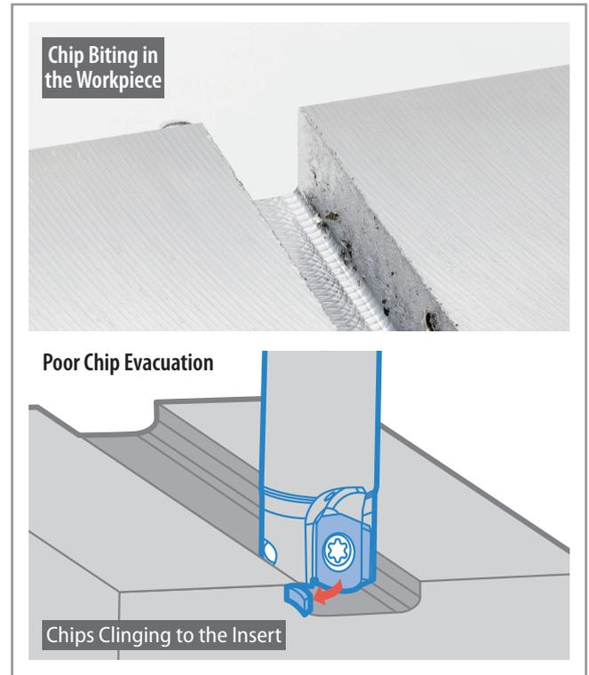
Cutting Conditions: Cutter Dia.  $D_c = \varnothing 10$  mm,  $V_c = 120$  m/min,  $f_z = 0.6$  mm/t,  $a_p = 0.4$  mm (25 Passes) Total 10 mm, Dry Workpiece: S5400
